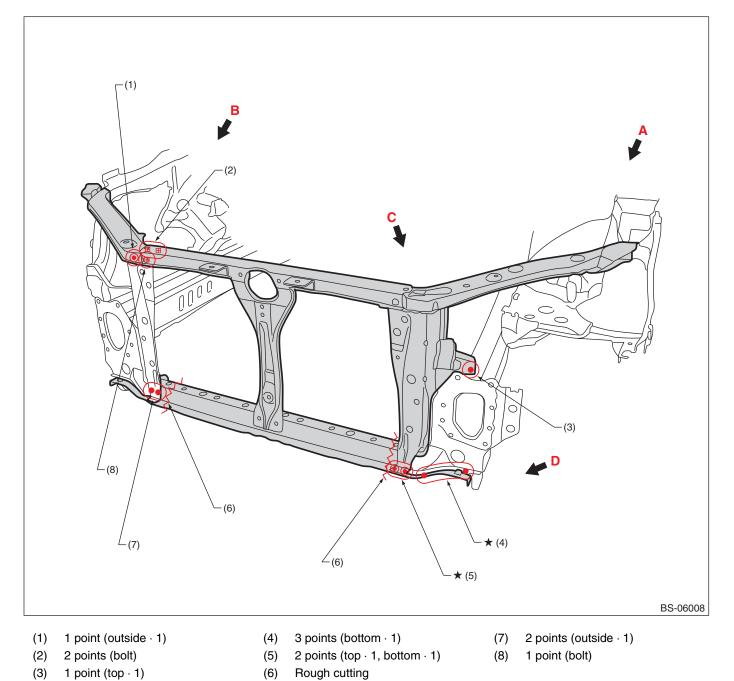
For locations marked by " $\star$ ": the welding method and the number of welding points are the same on the left and the right.
