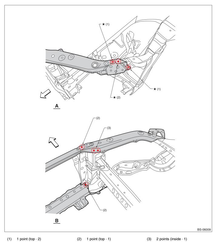
For locations marked by " $\star$ ": the welding method and the number of welding points are the same on the left and the right.
